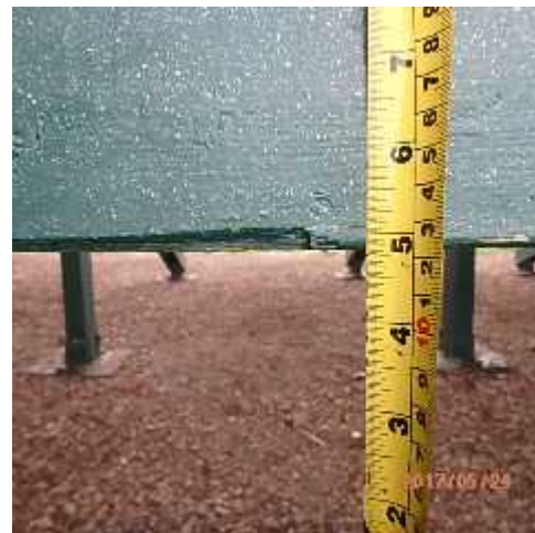
Photo 50: Maximum gap allowed is 4".
